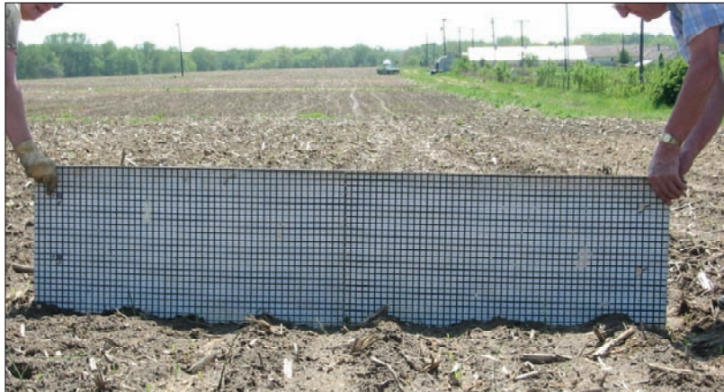
Figure 4-3 The 2 m grid board placed in soil surface for characterizing the surface roughness.
